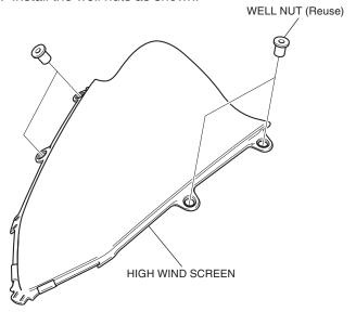
14. Install the high wind screen as shown.
