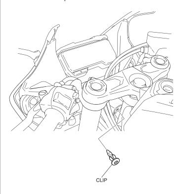
6. Remove the meter as shown.
