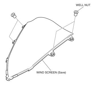
13. Install the well nuts as shown.
