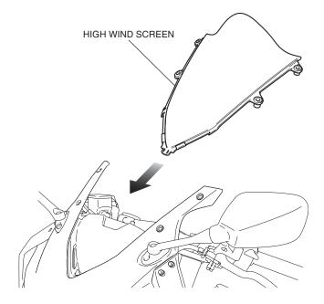
15. Install the parts as shown.
