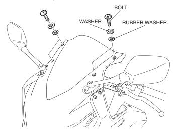
2. Remove the wind screen as shown.
